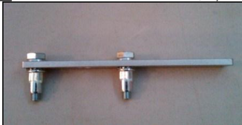
Picture I: The Rivet-nut install tool with 2 Gold/Silver Rivet-nuts on it, ready to be installed.
