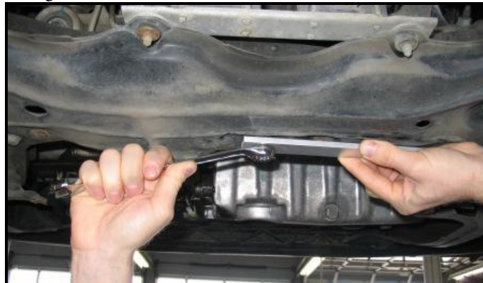
Picture G: Showing how to install the Rivet-nut into the center hole on the lower sub frame.
