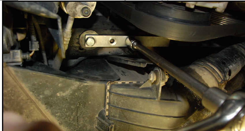
Picture K: Install tool with 2 Rivet-nuts being installed by your driver with wobble head extension.
